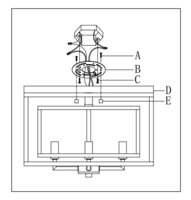
Line art shown may not exactly match the fixture enclosed. However, the installations do apply to this fixture. ITEM NO: 457F-CH-MB 457F-OBR-BRZ
